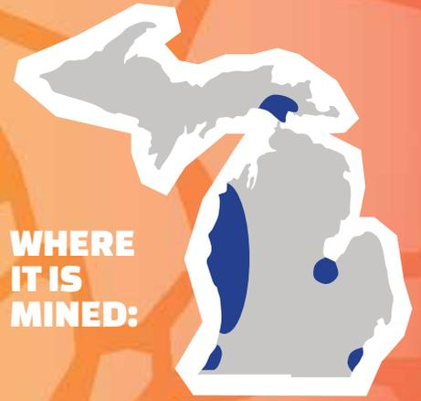
Silica Sand is quartz that over time has been broken down into tiny granules. In Michigan, Silica Sand is most commonly surface-mined in open pit operations. It is found nearly everywhere across the state, with most of the mining operations focused on the west coast near Lake Michigan.
