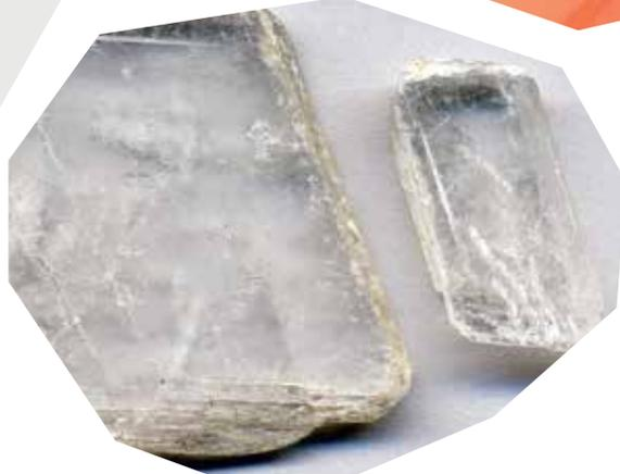
**USES:** Gypsum is used in fertilizer, drywall, sheetrock, cement and plaster of Paris. It is also used in toothpaste and make-up.
