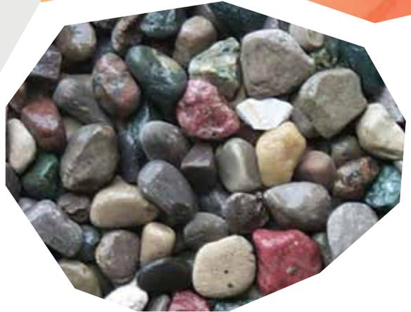
**USES:** Natural Stone or Gravel is primarily used in construction. You can use it to build roads by mixing it with cement to produce concrete or with liquid asphalt to pave the roads we use every day. When Natural Stone is mechanically crushed it will have sharp edges and can be used to build roads with improved skid resistance.
