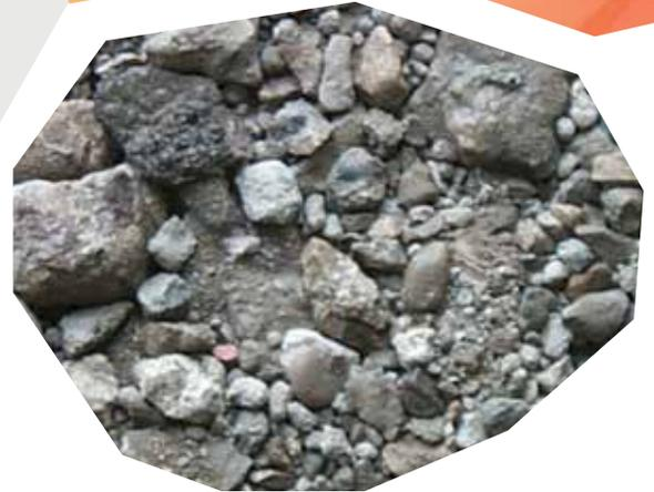
**USES:** Recycled Concrete is mainly used in the base mixture for roads and to keep areas from eroding.
